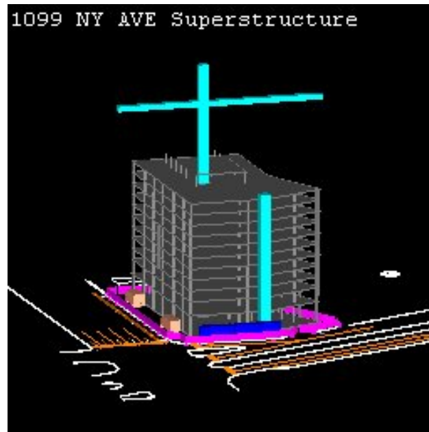
Figure B.4 Construction of the superstructure is complete. The material hoist has been installed as well.
